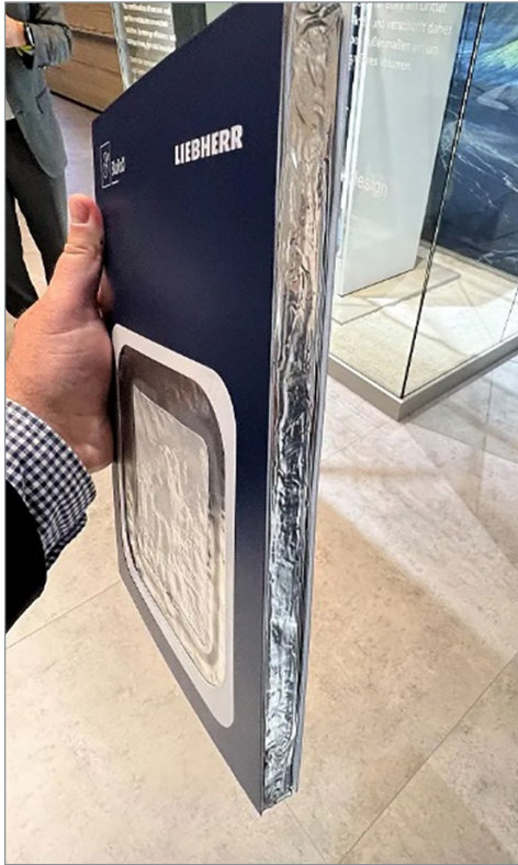
Figure 6 • Outer (left) and inner (right) view of a perlite-core vacuum insulation panel.
